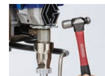
1) Loosen the clamping nut
